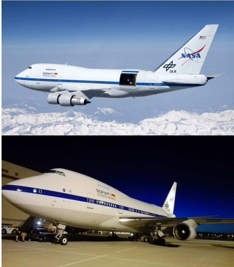
Fig. 4-10: The joint DLR and NASA SOFIA observatory flying with the telescope door wide open (top). The bottom panel shows SOFIA on the tarmac of NASA Armstrong (Palmdale) about an hour before take-off for an observing night.
