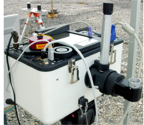
Fig. 3-28: The D&P Model 102 Field FTIR.
