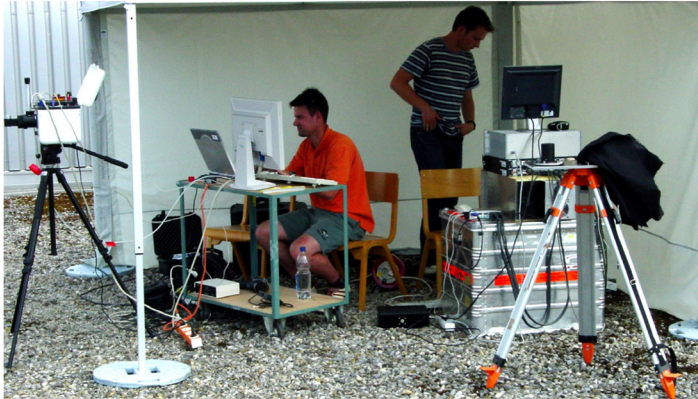
Fig. 3-27: Planned experimental set-up during the SAMUM 2 field campaign: IMF FTIR (left) and equipment from the University of Mainz (right).
